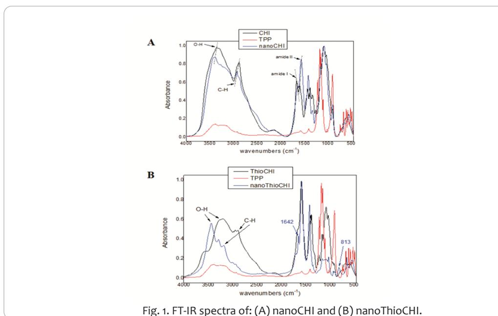
Fig. 1. FT-IR spectra of: (A) nanoCHI and (B) nanoThioCHI.
