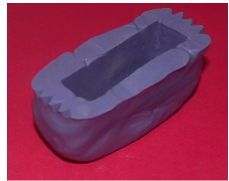
Figure 2 The future mould space for the resin.
