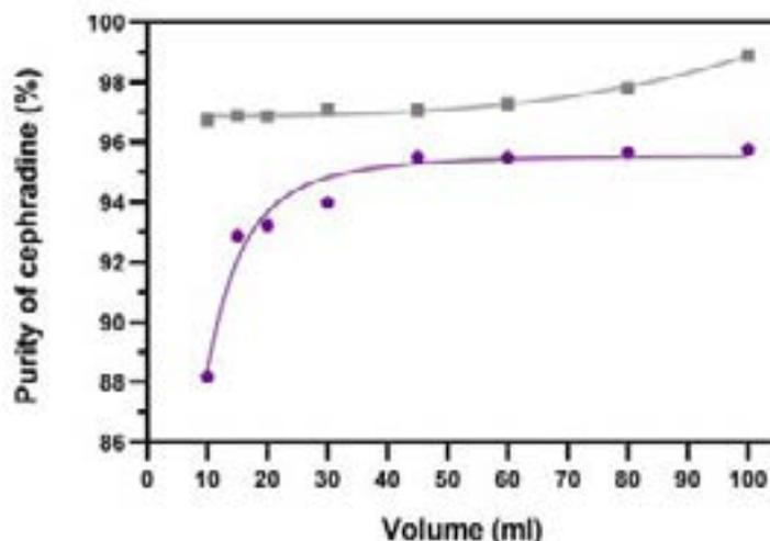
Fig. 4 Effect of volume on the purity of cephradine during purification process based on solubility
