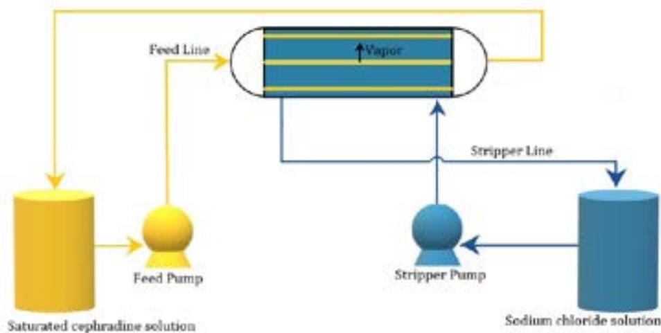
Fig. 1: Flow outline of OD unit with HFM for cephradine solution concentration
