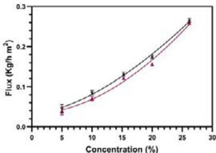
Fig. 6 Effect of stripping solution concentration on flux during osmotic distillation (Ambient temperature, feed flow rate:  $0.108\text{m}^3\text{h}^{-1}$  and  $0.048\text{m}^3\text{h}^{-1}$ )
