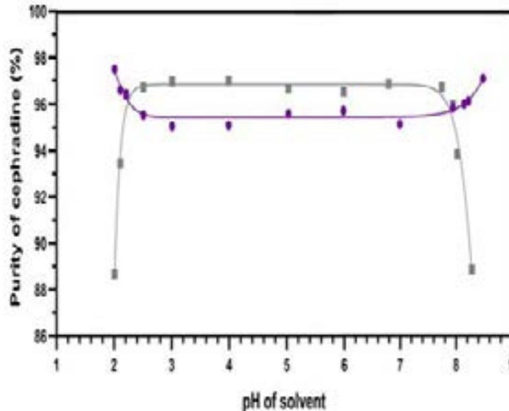
Fig. 3 Effect of pH on the purity of cephradine during purification process based on solubility
