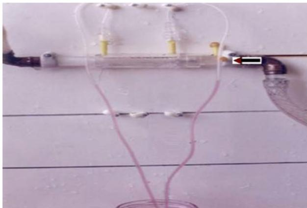
Figure 4. The G-C model measuring the negative pressure in C with manometers sucking water from a jar 30 cm below.
