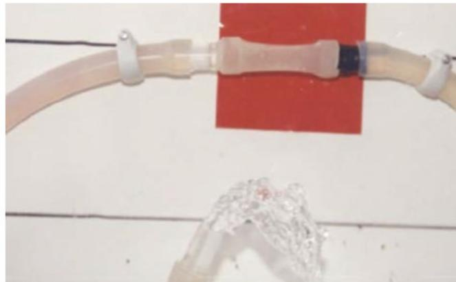
Figure 3. The G-Tube enclosed in a rubber chamber (C) which is sucked in as water passes through the G tube indicating net negative pressure in C.
