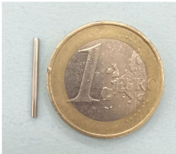
Figure 6) Biopsy punch without plastic body before incorporation into the stamp
