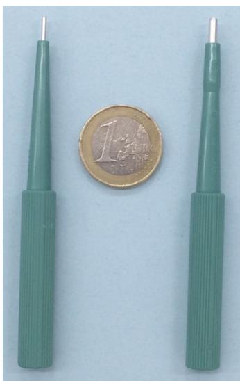
. 2) Standard biopsy punch for the first part of the experiment. Left 1 mm and right 2 mm biopsy diameter
